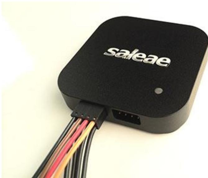
Note that the test lead color matches the channels in the software. The colors reflect the resistor color code for numbers 0–7. The numerical channel number is on the white heat shrink at the ends of the leads. The lead ends are terminated with a Molex 0016020086 crimp connector for connection to typical .100-inch spaced headers/pins. The 2x4 plastic housing is Molex 0022552081.
